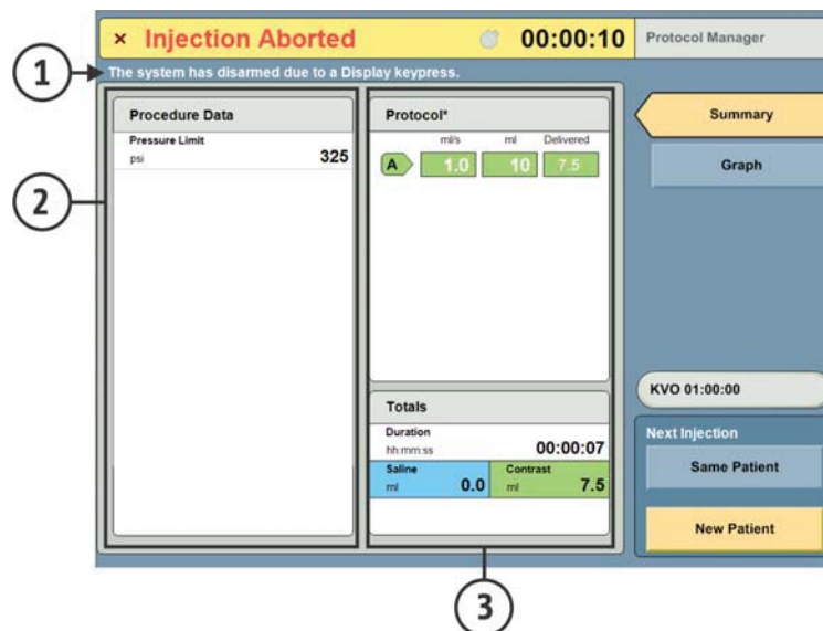
Figure 13 - 3: Injection Complete - Injection Aborted
